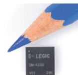
LEGIC advant reader chip SM-4200 size 8x8 mm (1:1 illustration)
